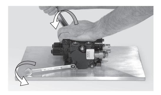
Install auxiliary valves and plugs and torque to proper specifications.
