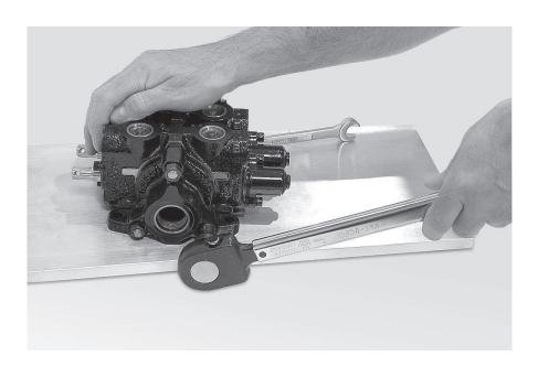
A noteworthy technique is to position the open-end or box type wrench over the nut so rotation during torquing operation is prevented by wrench making contact with working surface.
