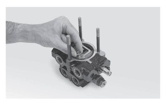
Repeat this procedure for additional spool sections. Special care must be taken to ensure o-ring and / or load check spring are not pinched between sections during assembly. Lastly, position the outlet section over the last spool section as shown.
