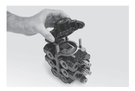
After hand-tightening all three tie rod nuts, position the valve assembly with the mounting feet on a smooth and flat working surface. To ensure proper alignment of entire valve assembly, apply a downward pressure to the inlet and outlet sections prior to torquing tie rod nuts.
