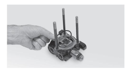
Place first spool section over inlet section with o-ring groove facing upward and install o-ring into groove. Special care must be taken to ensure o-ring has been completely installed in groove. Install load check poppet into load check cavity as shown (nose-first into cavity). Once load check poppet has been properly installed, place load check spring in hollow cavity inside check poppet.
